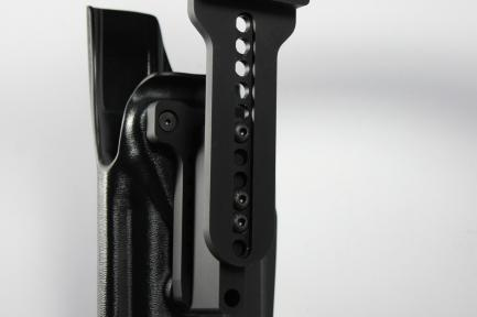
If choosing Forward or Reverse Cant, the spacer will need to have the letter D near the top of the Holster Bracket. In this configuration, you will only use two 10/32 screws. The screws will be installed in holes D and B OR D and C depending on the amount of cant desired. If using a minimum amount of cant you will use two adjacent columns of the
